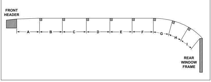
Start from the rear edge of the windshield header and measure to the FRONT edge of the first bow. Then measure from the FRONT edge of the first bow to the FRONT edge of the second bow, etc. Measure all the way to the wood over the rear window. Your car may not have this many bows.
